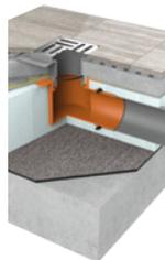
Combination of a TOPWET balcony outlet with an integrated sleeve for screed insulation and a balcony attachment with a stainless steel grid adjusted on site as required.
