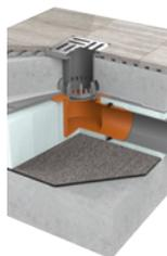
Combination of a TOPWET balcony outlet with an integrated sleeve and a balcony attachment with a stainless steel grid and a drainage ring used for water drainage from the main hydro-insulation layer.
